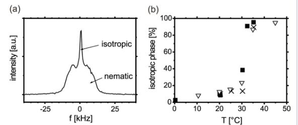
(a)  $^1\text{H}$  NMR solid echo spectrum, taken at  $30\text{ }^\circ\text{C}$  (particle size:  $R = 430\text{ nm}$ ). (b) The temperature dependence of the fraction of the isotropic phase for different particle sizes.  $\blacksquare$ :  $R = 120\text{ nm}$ ;  $\nabla$ :  $R = 430\text{ nm}$ ;  $\times$ :  $R = 780\text{ nm}$ . Weight fraction of colloids: 15%.
