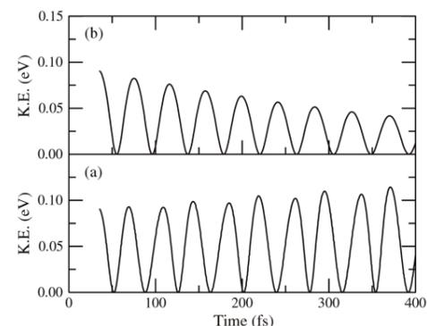
The variation of the ionic kinetic energy of the mobile atom with time for a bias of (a)  $0.1 \text{ V}$  and (b)  $1.0 \text{ V}$ . The device contains 3 atoms, and the leads 16 atoms. The initial temperature is about  $600 \text{ K}$ .
