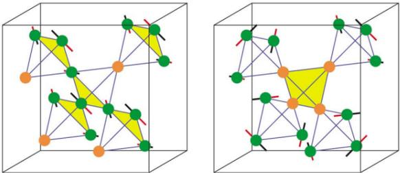
Comparison of (left) the 1- $k$  structure and (right) its 4- $k$  variant. In each structure the four  $\text{Gd}^{3+}$  ions coloured orange are shown as carrying no thermally averaged moment. The phase transition at  $T = 0.7$  K involves weak ordering of these four spins and a small canting of the remaining spins away from the positions shown. At  $T \ll 0.7$  K, only these ions carry a disordered spin component.
