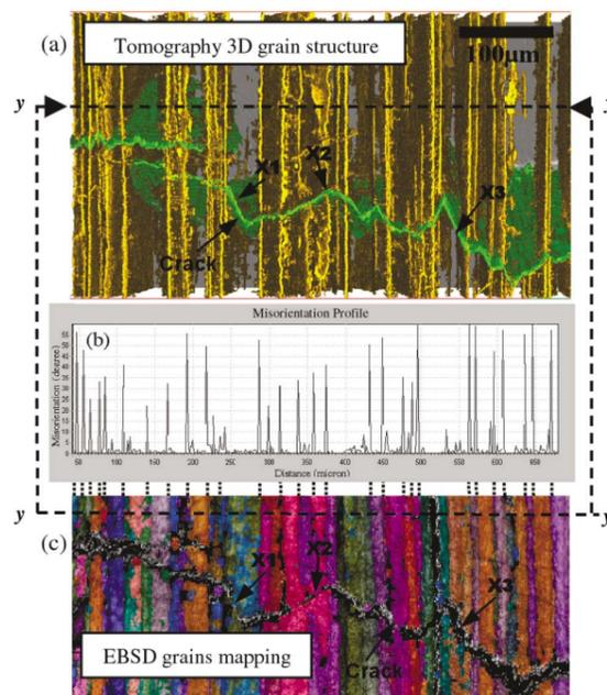
Comparison of the EBSD grains map and tomography data: (a) 3D reconstruction of grain boundaries (yellow) and the crack (green), (b) grain misorientation data from the EBSD data in (c), along the line  $y$ - $y$ , and (c) an EBSD orientation map of the sample at the front plane of the image (a).
