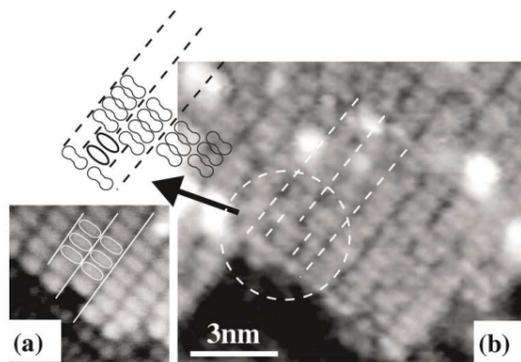
Detailed comparison between (a) a typical thermally annealed surface and (b) an electron-irradiated surface after ion bombardment. Out-of-phase dimers are seen in the broken circle.
