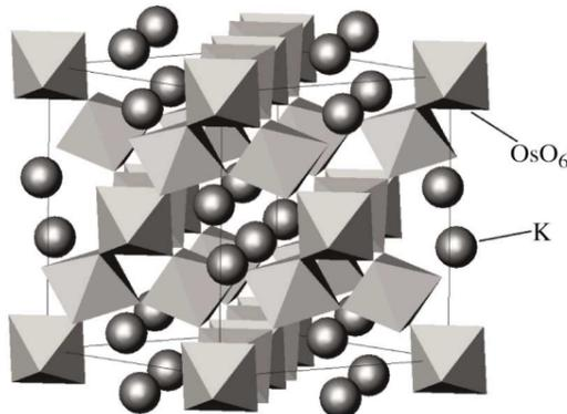
Probable crystal structure for  $\text{KOs}_2\text{O}_6$ . K, Os and O atoms occupy the 8b, 16c and 48f sites in the space group  $Fd\bar{3}m$ , respectively.
