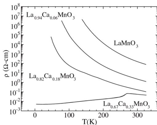
Temperature dependence of the resistivity for class I  $\text{La}_{1-x}\text{Ca}_x\text{MnO}_3$  for  $x = 0.0, 0.06, 0.18$  and  $0.33$ .
