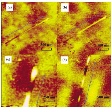
Magnetic force micrographs of a multiwalled nanotube lying on a magnetite substrate obtained in the amplitude mode with a low-moment, permalloy-coated tip.
