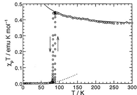
The magnetic susceptibility of galvanoxyl. Ferromagnetic interactions dominate above the phase transition at 85 K. The high-temperature behaviour fits to a one-dimensional ferromagnetic Heisenberg model and the low-temperature behaviour fits to a singlet-triplet model.
