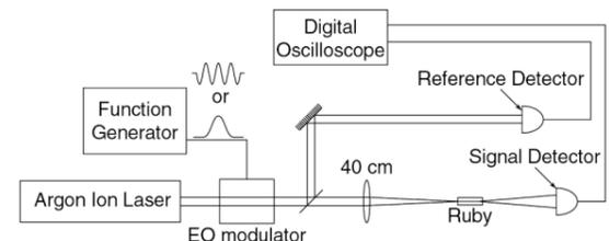
The experimental setup used to observe slow light in ruby.
