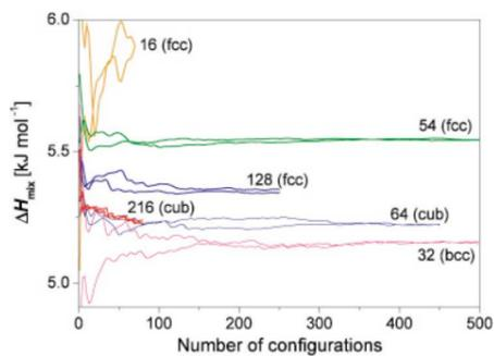
Calculated values of  $\Delta H_{mix}$  ( $\text{kJ mol}^{-1}$ ) for a 50/50 MnO-MgO composition at 1000 K as a function of supercell size and number of configurations. The number attached to each curve denotes the total number of atoms in each supercell.
