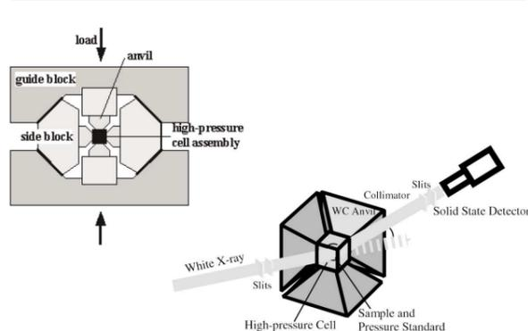
A schematic illustration of the in situ x-ray diffraction system combined with a DIA type multi-anvil high-pressure apparatus.
