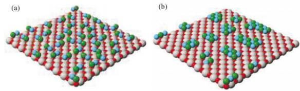
Evolution of BaO islands on the (100) surface of BaO. (a) Starting configuration; (b) after 380 ns simulation at 1000 K.
