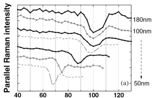
Parallel Raman intensity ( $I_{||}$ ) as a function of  $T$  of polystyrene for different film thicknesses going from 180 to 50 nm. A distinct crossover is observed below a specific thickness, which depends on the molecular weight.
