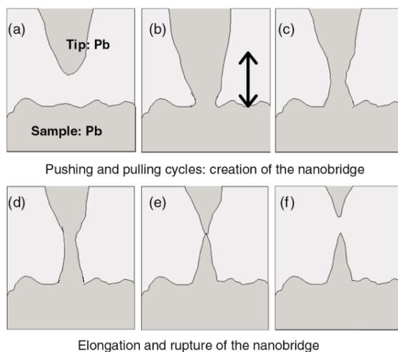
Sketch of the nanobridge fabrication process. Frames (a)-(f) illustrate different stages of the process: (a) tip and sample in tunnelling regime; (b) the tip is pressed against the substrate, both electrodes deform plastically and form a connective neck; (c)-(e) indentation-retraction cycles produce a plastic elongation of the neck; (f) the rupture of the nanobridge takes place.
