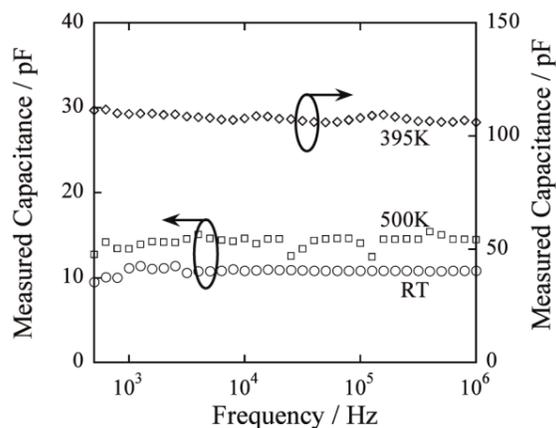
The frequency dependence of the capacitance measured at three different temperatures for thin  $\text{BaTiO}_3$  lamellae. All lamellae investigated showed the distinct lack of spectral dependence illustrated here. Strong temperature dependence is, however, evident.
