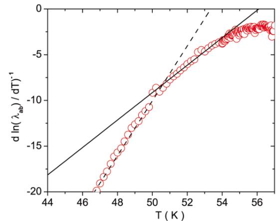
$(d \ln \lambda_{ab} / dT)^{-1}$  with  $\lambda_{ab}$  in  $\mu\text{m}$  versus  $T$  for  $\text{YBa}_2\text{Cu}_3\text{O}_{6.59}$ . The straight line with slope  $1/\nu \approx 3/2$  corresponds to charged criticality with  $T_c = 56.1$  K, while the dashed line indicates the intermediate 3D XY critical behaviour with slope  $2/\nu \approx 3$ .
