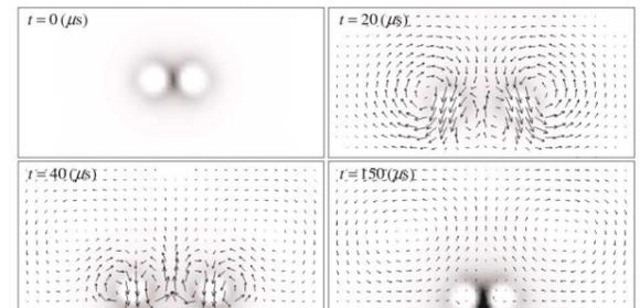
Snapshots of the process of the electrophoretic deposition of two charged particles placed between the electrodes. The density plot represents the counterion concentration. The arrows indicate the velocity field. The electrodes are separated by  $310 \text{ nm}$  ( $d = 310 \text{ nm}$ ). The applied voltage is  $V = 100 \text{ mV}$ . The average concentration of the added salt is  $10^{-2} \text{ M}$ .
