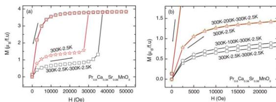
(a) Isothermal  $M(H)$  curves of  $\text{Pr}_{0.6}\text{Ca}_{0.34}\text{Sr}_{0.06}\text{MnO}_3$  registered at  $T = 2.5$  K after different thermal cyclings (300 K-2.5 K and 300 K-2.5 K-300 K-2.5 K). (b) The enlargement of the field increasing branches of the  $M(H)$  curves after different thermal cyclings. The arrows indicate the magnetic field increasing and decreasing branches.
