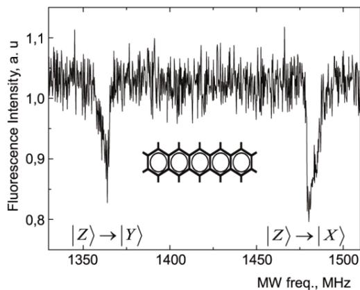
The ODMR spectrum of a single pentacene molecule. The inset shows the chemical structure of pentacene.
