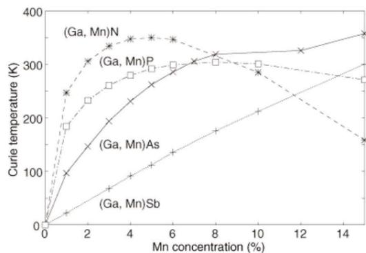
Curie temperatures of (Ga, Mn)N, (Ga, Mn)P, (Ga, Mn)As and (Ga, Mn)Sb calculated from first principles in the mean field approximation. [from Exchange interactions in diluted magnetic semiconductors, K Sato, P H Dederichs, H Katayama-Yoshida and J Kudrnovský, J. Phys.: Condens. Matter 16 S5491-S5497]
