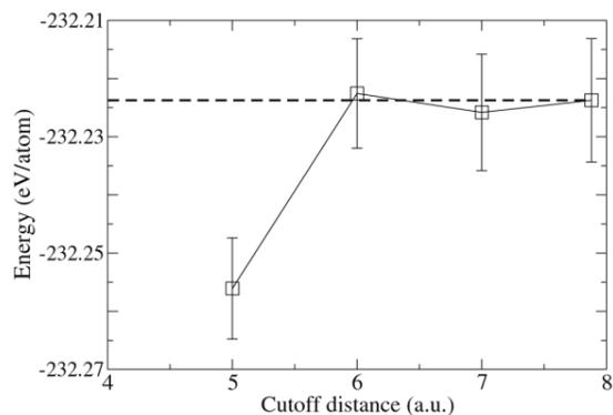
Convergence of linear-scaling diffusion Monte Carlo total energy per atom to the value obtained with extended orbitals for bulk MgO. Open squares with statistical error bars: the present method with cubic cut-off. The dashed line shows the result with extended orbitals. This shows that the energy appears to be converged within  $\sim 10$  meV/atom for a cut-off radius of 6 au.
