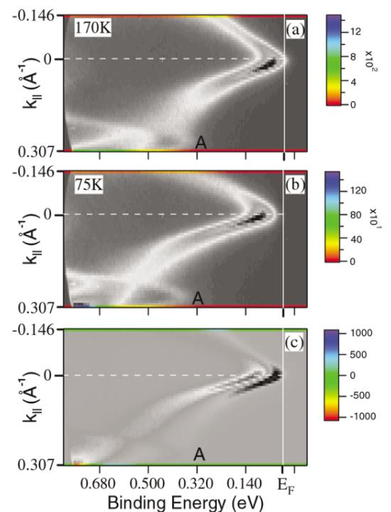
Intensity maps of the density of states of  $ZrTe_5$  acquired along the  $\Gamma$ -X high symmetry direction for (a)  $T = 170$  K and (b)  $T = 75$  K, and (c) an intensity difference map between the maps in (a) and (b)
