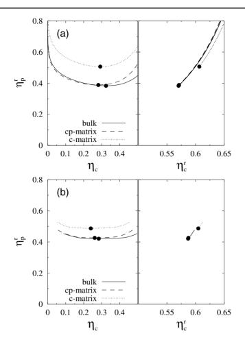
**Figure 5.** Demixing phase diagram for the model colloid–polymer mixture in contact with different HS matrices as a function of  $\eta_c$ ,  $\eta_p^r$  (left panels) and  $\eta_c^r$ ,  $\eta_p^r$  (right panels) for  $\eta_m = 0.05$  and size ratios q = 0.3,  $\sigma_m/\sigma_c = 1$ . Tielines between coexisting phases are horizontal in the left panels. (a) DFT result, (b) ORPA result.
